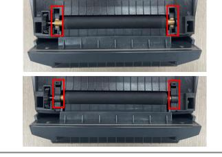
Place the bottom of the Printer face the front. Press the Hooks (red circles) toward the inner side to remove the Cover DIP. Then, shape the Auto Cutter Wire and Auto Cutter GND Wire as shown below. imes Be careful to avoid tangling with other wires when shaping. Cover DIP **Auto Cutter Wire**
